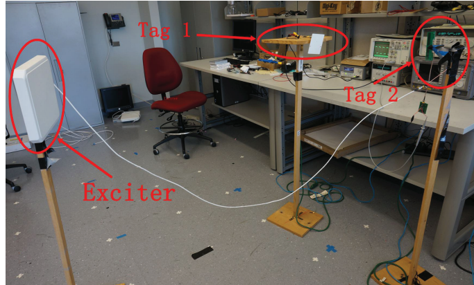
Figure 2.13: The experimental setup composed of one exciter and two tags.
