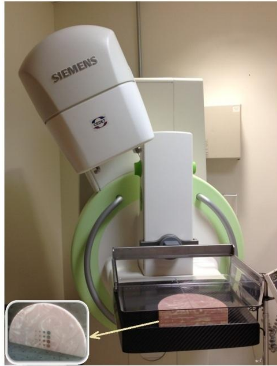
Figure 6.2. The Siemens Mammomat Inspiration DBT unit is shown with the phantom situated for acquisition. The compression paddle sits atop the phantom, and the phantom sits directly atop the carbon-fiber detector cover. The inset shows the slab of the phantom with the iodine inserts. The gantry is shown at its extreme angle of 25 degrees.
