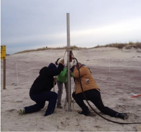
Figure 12: (Left) The sediment core is being drilled into the ground by the power from the motor and the downward force of three ropes, evenly spaced around the sediment core.
