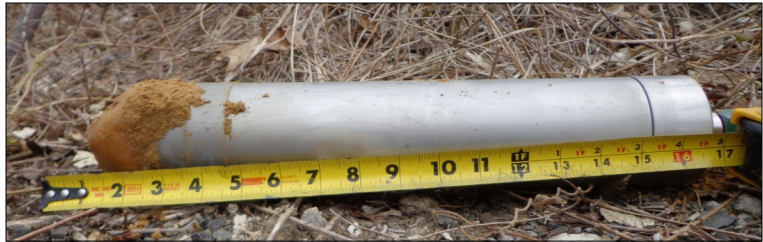
(Fig 2.1) Image of split spoon corer, with a rock protruding from the head of the corer. Only the core sampler is shown.
