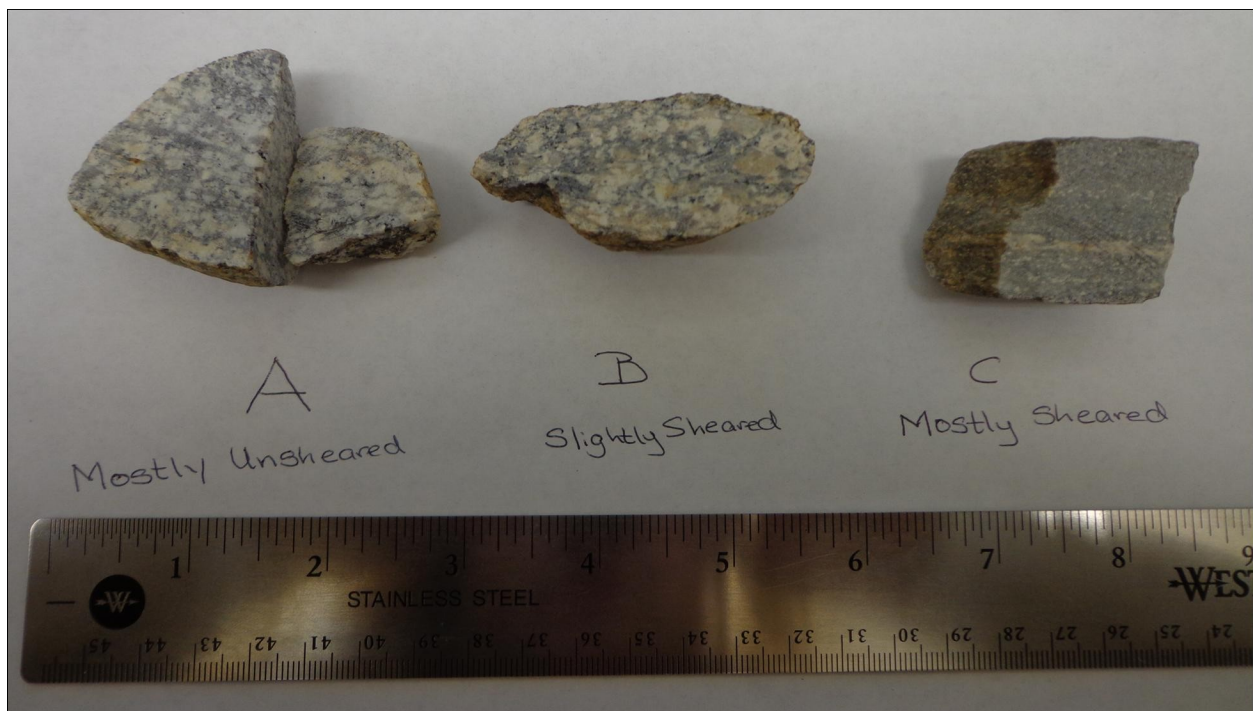
(Fig 2.3) The three specimens of granite gneisses collected on the Stony Brook campus, used for whole rock grinding analysis.
