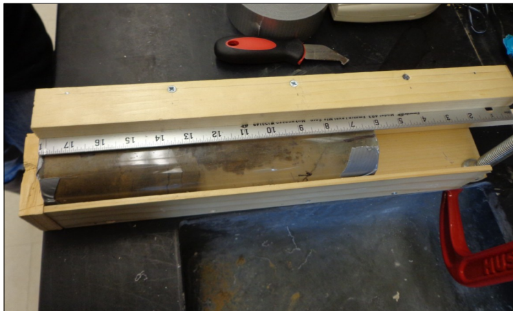
(Fig 2.2) Jig used to open the core sleeves from the split spoon corer. Plexiglas cutter visible to the top center of image.
