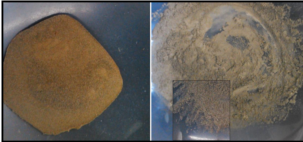
Figure 5-18 Image of MH-amorphous precipitated onto <63 μm flood basalt unground (left) and ground (right). The inset on the right shows the ground, uncoated flood basalt.
