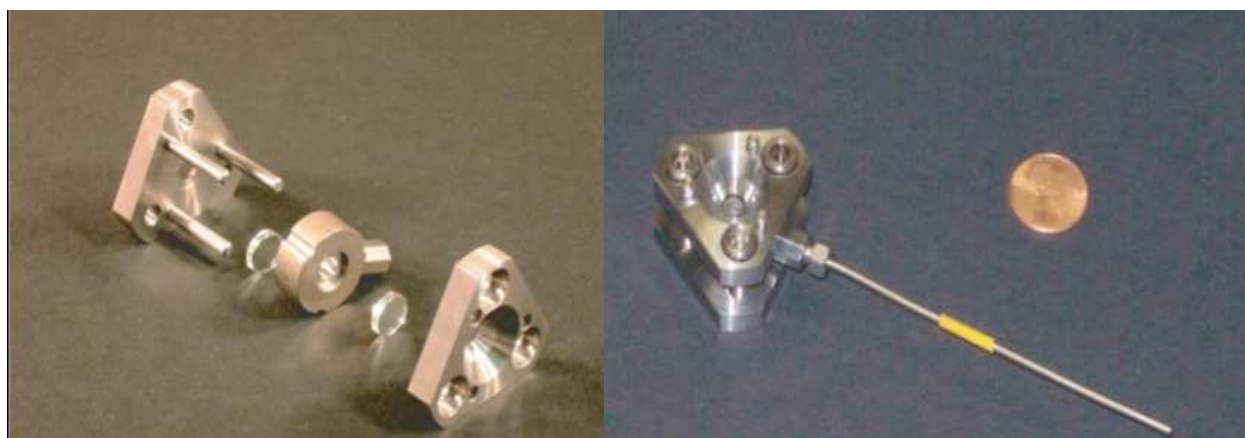
(Fig. 2.3.1) A photo of the microreaction cell designed by Diefenbacher (Whitfield et al., 2008). It was designed to for reactions involving any combination of fluid-fluid, solid-fluid, solid-gas, and fluid-gas systems (Diefenbacher et al., 2005)
