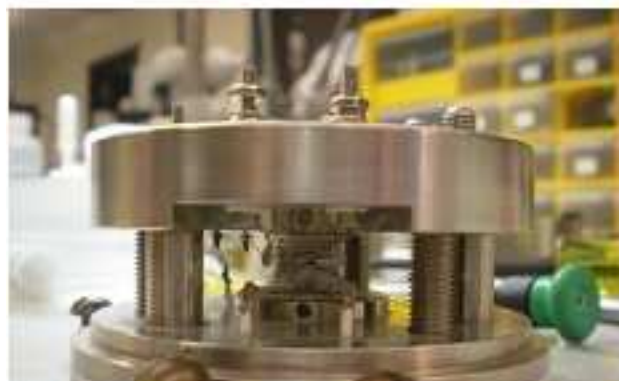
(Fig. 2.1.1) In 1993, this Hydrothermal Diamond Anvil Cell, called the Bassett-type Cell, was invented (Bassett et al., 1993)
