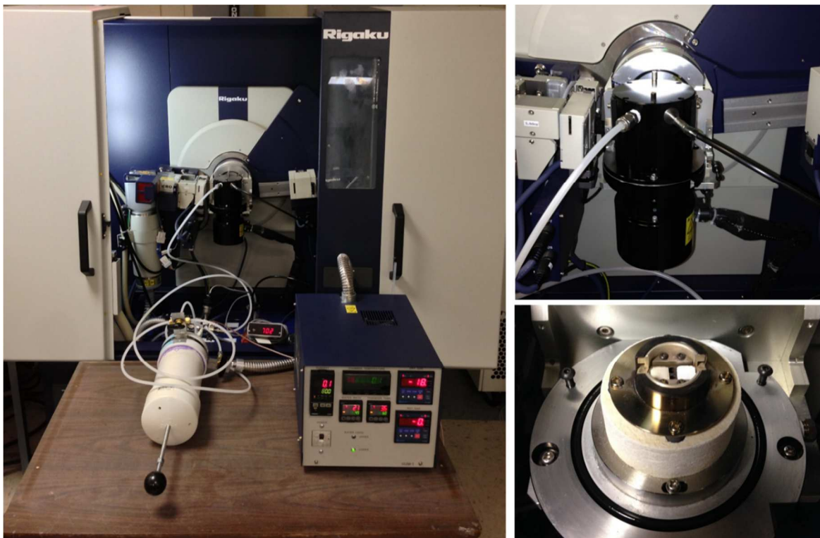
Figure 1. (Left) Photo of complete XRD-DSC system. (Top right) XRD-DSC stage with sealing cap. (Bottom right) XRD-DSC attachment without cap showing the Al 2 O 3 standard and sample powder on aluminum pans.
