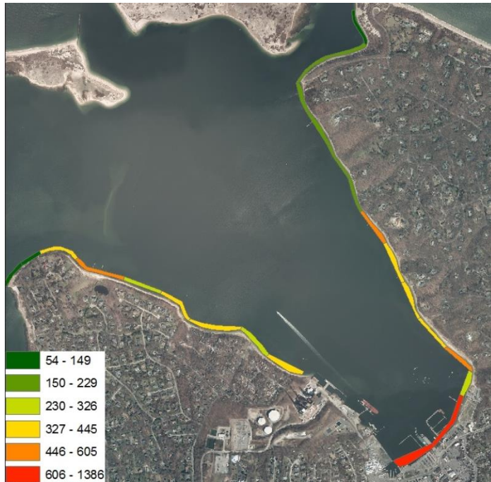
Figure 35 SGD total for harbor shoreline. Each polygon represents the half-way point between radon measurements, and is comprised of 11m of intertidal area plus 9m of sub-tidal area.
