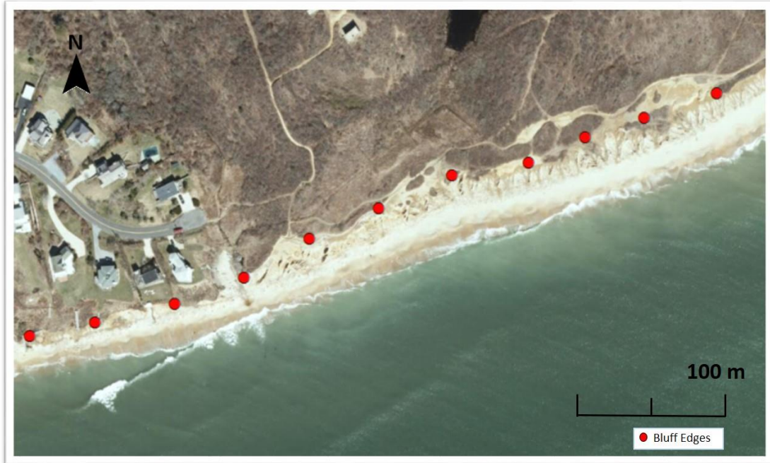
Figure 3. 5. Bluff edge points (red points) along the bluff on 2013 modern ortho-images.
