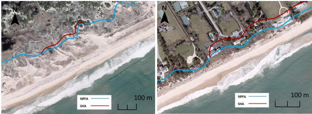
Figure 3. 1. Two type of (Coastal Erosion Hazard Area) CEHA, Natural Protective Feature Area (NPFA) line and Structural Hazard Area (SHA) line.
