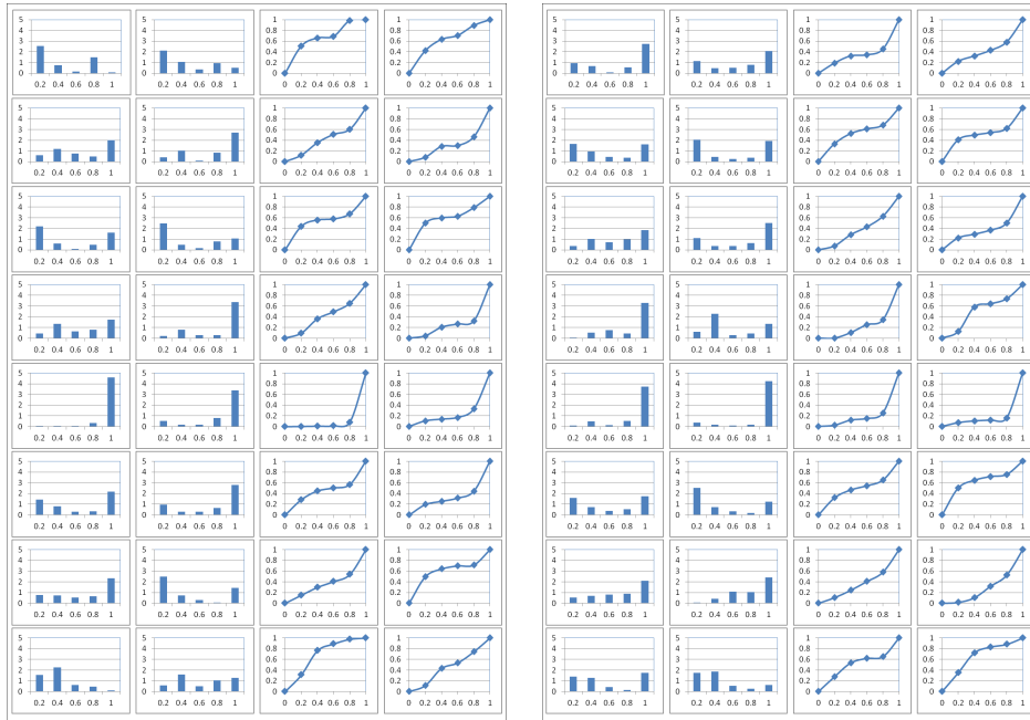
Figure 3.2: Spatial array of heavy fluid concentrations at t = 50 , for z in the midplane, as PDFs (bar graphs) and as CDFs (line graphs), Left: medium grid. Right: fine grid.
