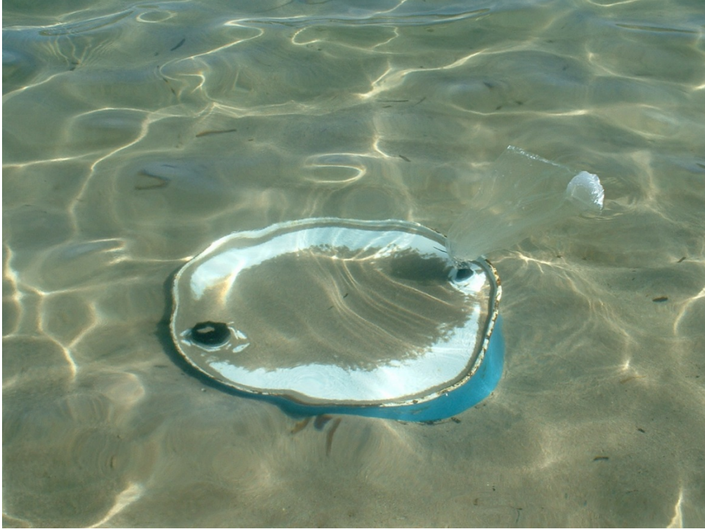
Figure 1.2. Photograph of seepage meter in-situ. Credit Ruth Coffey.
