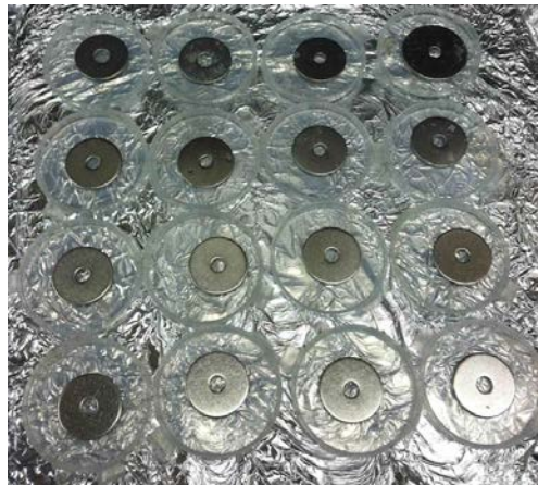
Figure 6.2 a) Disks used to hold sediment for oxic plug incubations; note that weights are covered by a uniform layer of paraffin wax. b) entire set up of oxic incubations c) a plug filled with sediment after being sampled from the incubation tank.
