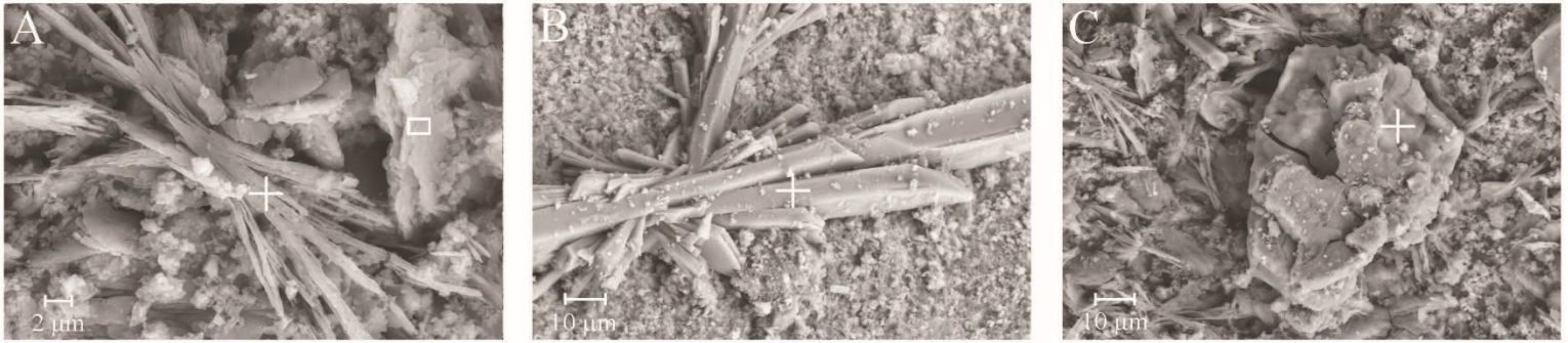
Figure 3-10: Scanning electron micrograph of BKSG-pH1 displaying A) cement rich in S, Si and Al (cross) and plates of Na-Al-sulfate (square), B) elongated Ca-sulfate, and C) Fe-Mg-sulfate.
