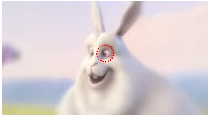
(b) Example of foveated compression (gaze focused on eye of the rabbit)
