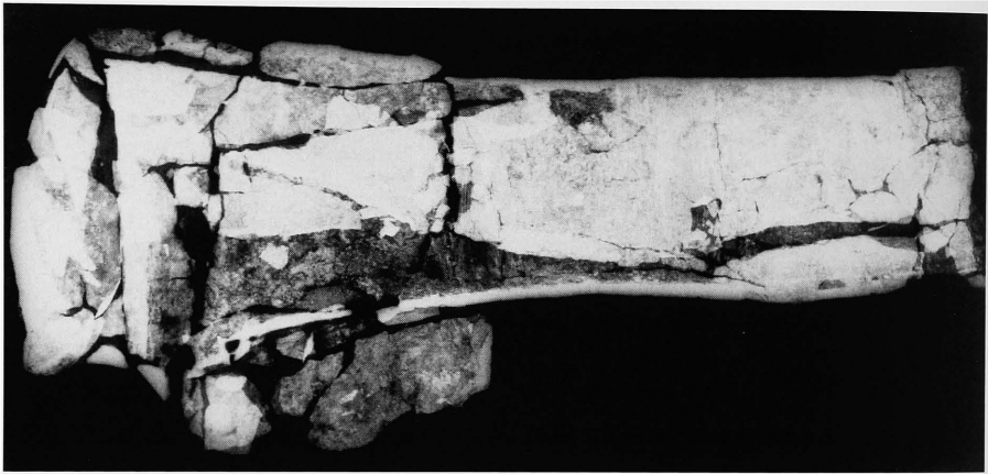
Plate 12. Conventional X-ray of the rear section of the yoke. The thickened metal of the folded and overlapped edges of the sheet can be seen along the bottom of the yoke. The folded back edge of the sheathing and the silver cap covering the terminal are also visible. No tacks or nails can be seen. (Courtesy Hospital of the University of Pennsylvania, Department of Radiology, 1994.)
