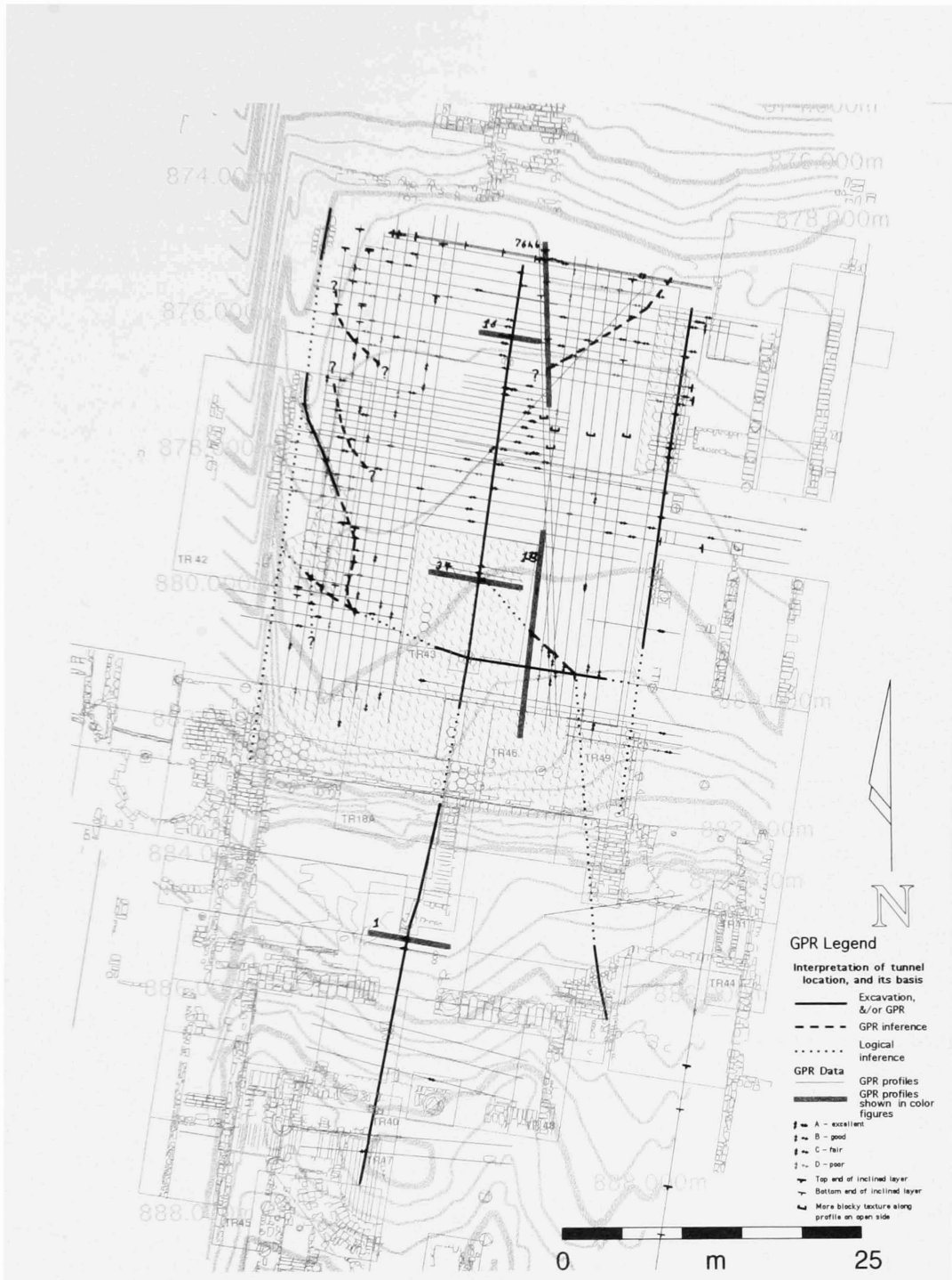
Figure 4.11. Map showing GPR data and interpretation superimposed upon architectural features and topographic contours (surveying by Loa P. Traxler and Paul C. Zimmerman). The straight gray lines represent GPR profiles. Profiles in the orthogonal grid on the Lower Temenos have been precisely located by survey. The locations of some other profiles have also been determined by survey, but for others the location is only approximate. The five wider gray lines represent the correspondingly numbered profiles in Color Plate 9. Double-headed arrows with varying degrees of darkness, as shown in the legend, indicate four qualities of hyperbola reflections. Symbols indicating differences in general subsurface radar characteristics as well as symbols indicating inclined layers are also plotted (see text for more detail). Tunnels of the Canalization System are indicated in dark lines, solid, dashed or dotted depending upon our confidence in the feature and the method in which we inferred their locations. Those wishing further use of this GPR map and user-navigation may find a full-color digital copy on the CD-ROM archive.
