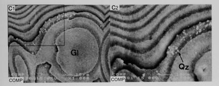
Fig. 15.18 External appearance of No. 1 and the results of structural analysis. a<sub>1</sub>: External appearance. The sample was extracted from the marked location in a<sub>1</sub>. b<sub>1</sub>: Macrostructure. c<sub>1</sub> and c<sub>2</sub>: Compositional images by EPMA. The analytical locations of c<sub>1</sub> and c<sub>2</sub> by EPMA are shown in b<sub>1</sub> and c<sub>1</sub>, respectively.
