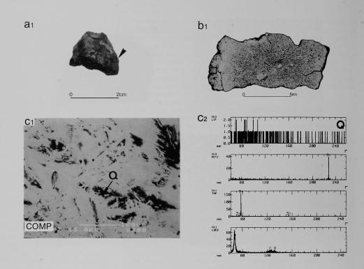
**Fig. 15.20 External appearance of No. 2 and the results of the metallographic analysis.**  $a_i$ : External appearance. The sample was extracted from the marked location in  $a_1$ .  $b_1$ : Macrostructure.  $c_1$ : Compositional image by EPMA.  $c_2$ : The result of the qualitative analysis of the Q area in  $c_1$ .
