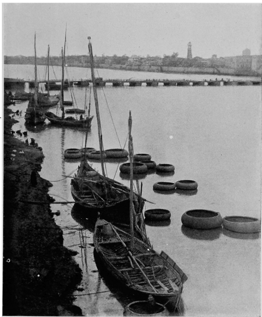
A Scene on the Tigris at Baghdad, showing characteristic native boats, the long turadas, and the round, pitch-smearred kufas, with bridge of boats beyond.
