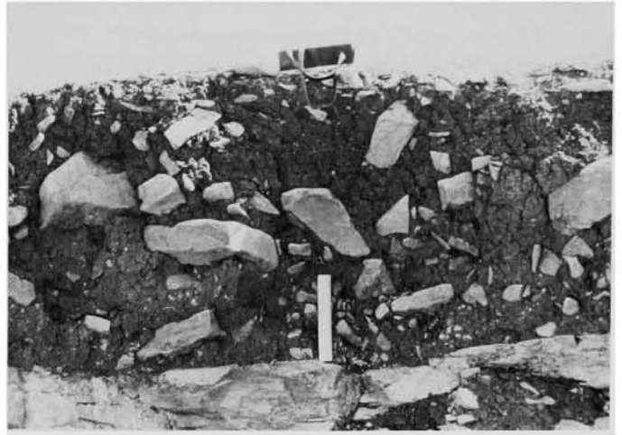
FIG. 16. Colluvium over limestone bedrock, consisting of fresh, angular limestone blocks set in matrix of colluviated terra rossa , near Toveh Latif, south-southeast of Kermanshah. 25 July 1975.
