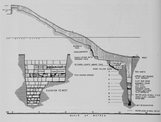
Fig. 12. East-west section through the citadel and quay walls, on the western side of the citadel.
