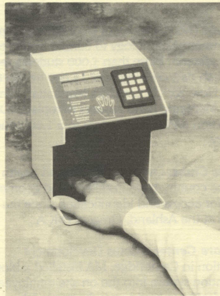
This ID3D Hand Key, hand-geometry, scanner from Recognition Systems, Inc. will be used as a major part of security at the 1996 Olympic Games in Atlanta, Georgia. Biometric Identification will help control access to the Olympic Village.
