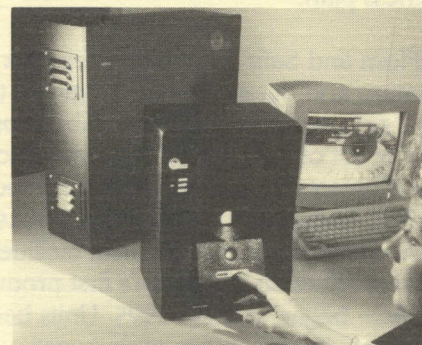
With over 400 identifiable characteristics, the iris offers one of the most accurate forms of Biometric Identification in the Auto ID industry. Shown here is the IriScan System 2000EAC.
