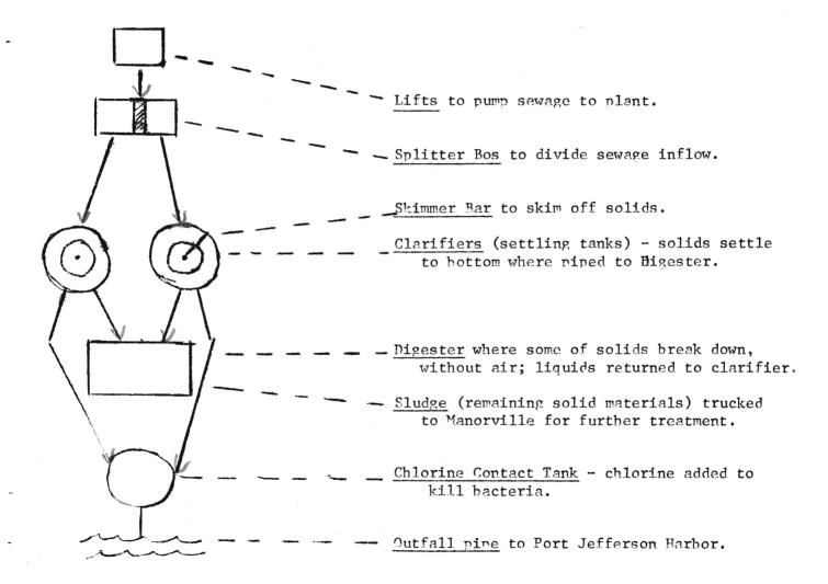
some of the dissolved and suspended solid materials from the liquid. After separation, some plants chlorinate the effluent, mandatory if it is discharged into a horbor, stream, river or lake. Sometimes the sludge is deposited in a land fill site. A primary plant cannot remove such sewage constitutents as nitrates, phosphates, pesticides, metals, grease, or tars.
