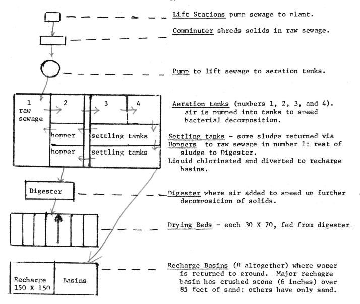
or piped to rivers, lakes or harbors. In the <u>activated sludge process</u> (which can be part of secondary treatment), compressed air is added to the sludge digesting stage t encourage additional bacterial action in breaking down the solids. As in primary trement plants, sludge is pumped to drying beds, removed for further treatment, or depos in land fill sites. Like primary treatment, also, secondary treatment is ineffective in removing nitrates, phosphates, metals, pesticides and tars.
